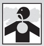
Serious injury or death could occur from inhaling gas engine exhaust which contains carbon monoxide- a poisonous gas that can kill you. You CAN NOT smell or see this gas.
