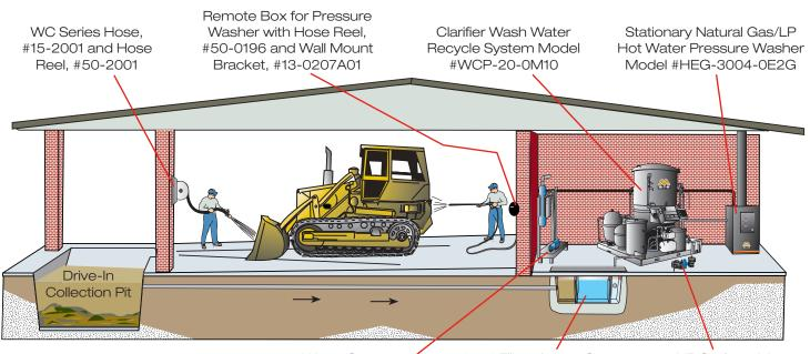
Water Cannon / Model #WC-100-0ME3 3' x 9' Fiberglass 3-Stage Collection Pit Model #12-0074 1.0 HP Surface-Mount Sump Pump Included with System, #3-0460
