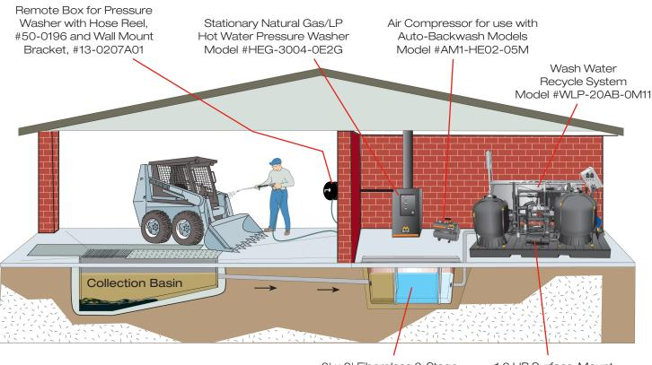
3' x 9' Fiberglass 3-Stage Collection Pit Model #12-0074 1.0 HP Surface-Mount Sump Pump Included with System, #3-0460
