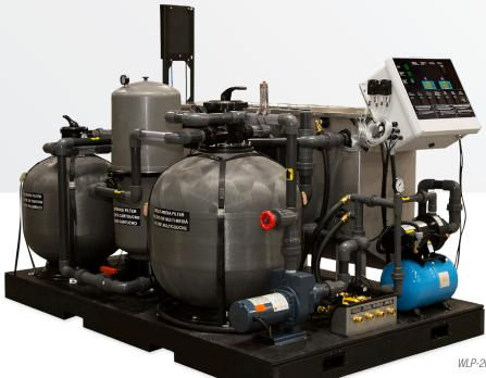
THESE RECYCLE SYSTEMS ARE DESIGNED TO REMOVE FREE HYDROCARBONS AND FILTER WATER TO BE SENT BACK THROUGH A PRESSURE WASHER. THEY FEATURE pH AND ORP INJECTION AND ARE DESIGNED WITH CORROSION-RESISTANT TANKS.
