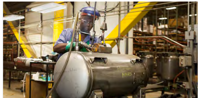
Advanced hydrostatic testing is performed on every air compressor vessel manufactured at Mi-T-M for strength and leaks
