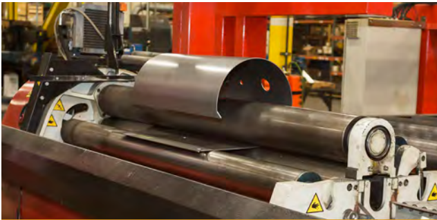
Automated CNC Roll Former rolls up to \frac{3}{16} -inch steel to create the shell of an air compressor vessel
