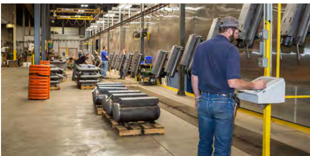
A 7-stage powder coating system applies superior finish that is harder and more durable than conventional paint
