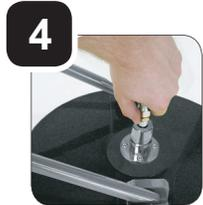
**4** Next, tighten the swivel end of the hose with a wrench into the top of the rotary head until snug.
