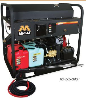
**Pump:** Belt drive triplex piston General or AR pump with ceramic plungers  $\cdot$  Factory preset unloader  $\cdot$  Forged brass manifold  $\cdot$  80-mesh, high volume, stainless-steel screen inlet water strainer
